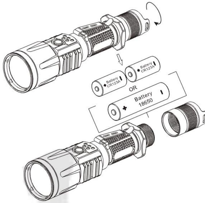
**ON/OFF:** Press the button on the tail cap. After a “click” is heard, the flashlight can be turned on or off.
